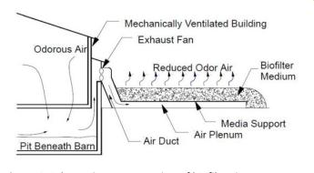
**Figure 6:** Schematic representation of biofiltration system where bacteria can be introduced into the media support for odor removal [125].
